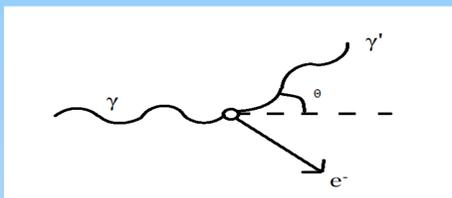
Figure 1: A diagram of Compton scattering
