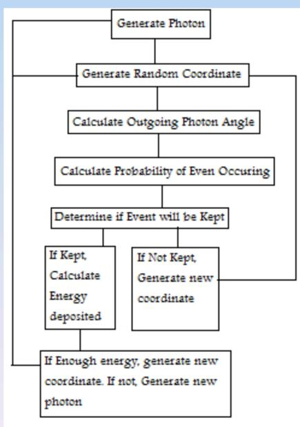
Figure 2. Flow chart showing the simulation steps.
