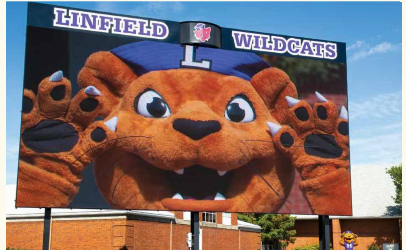
A new 8-ton video display at Maxwell Field is nearly 13 times larger than the previous video screen. With 15-millimeter LED resolution, the visual clarity is also 35% greater than the older version.
