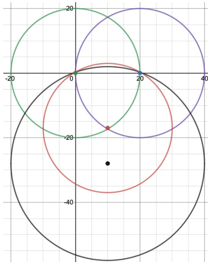
Figure 3: A red circle and dot representing a third drone and repeater have been added to the scenario from Figure 2 so that the EOC is able to communicate with the two furthest drones.
