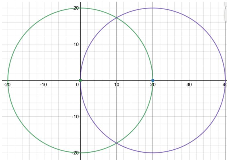
Figure 1: A drone is represented by a point and the circles represent the repeater range. The color of the circle correlates with the color of the drone it is associated with.
