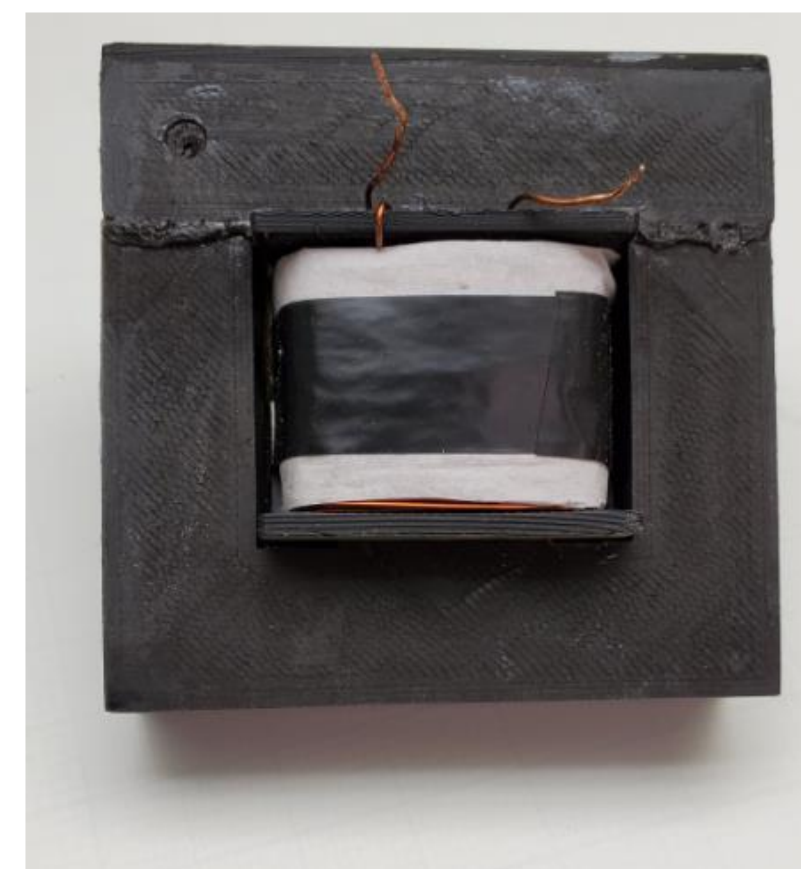
4) Coated Fe Core Core material was pressed and put into a 3-d printed case that provided strength and durability to protect the core.
