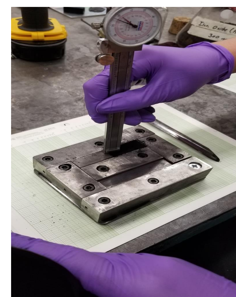
5) Core material being checked for consistency after being pressed.
