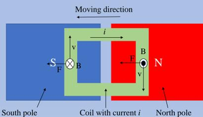
Figure.2: Diagram showing a basic part of a linear motor. Blue and red rectangles are south and north pole of permanent magnets. Green component is the coil of electromagnets. The current  $i$  in magnetic field generates force  $F$  as shown in the figure
