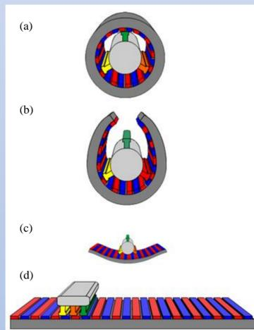
Figure.1: Diagram showing the process of a rotating motor expands to a linear motor. (a) a common structure of the rotating motor, (b) two transferring structures, (c) two transferring structures, (d) a practical structure of the linear motor. Image used with permission from Shcnibbi678.
