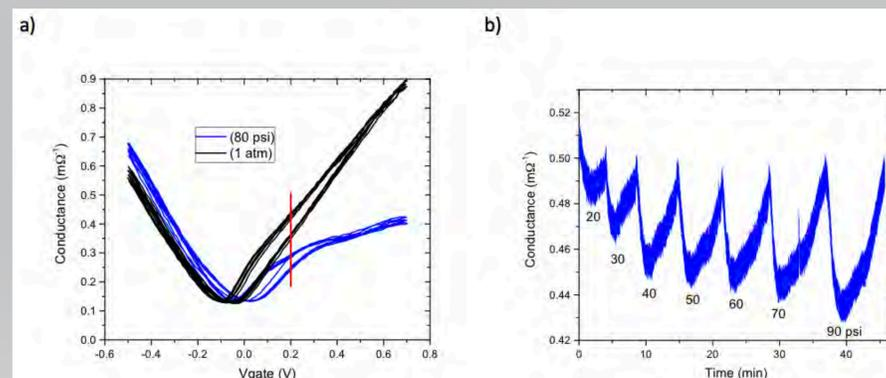
Figure 5: a) Plot of conductance vs gate voltage at two different pressures. b) The effect of pressure on the conductance of the GFET through several cycles of increasing pressure for  $V_g=0.2$  V.
