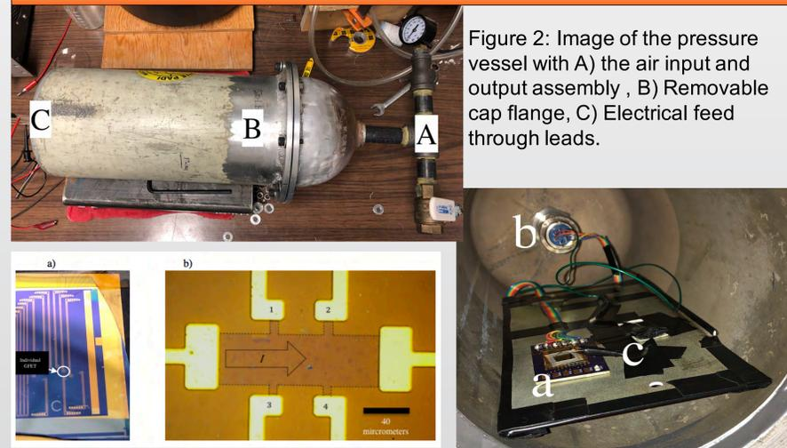
Figure 3: a) Photo of a GFET chip with nine individual GFETs. b) zoomed in view of a GFET wired for use. Current flows from the farthest left contact to the farthest right. Contacts 1 and two or 3 and 4 are used to measure resistance.
