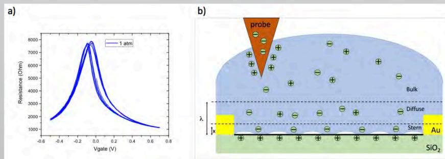
Figure 1: a) Plot of resistance within the graphene versus gate voltage. b) Schematic of a GFET in an electrolyte solution, with an external charge being applied by a probe. A double layer capacitance forms, consisting of the Stern and Diffuse layers.
