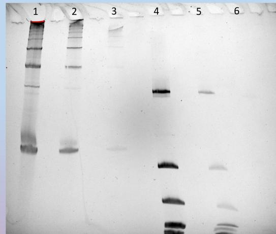
**Figure 3:** DNA and RNA on 5% PAGE run at 300 V for 3 hours, post stained with 1% SYBR Gold for 10 minutes. Lane 1 contains 3  $\mu$ L 0.28-6.6 kb RNA markers. Lane 2 contains 0.3  $\mu$ L RNA markers. Lane 3 contains 0.03  $\mu$ L RNA markers. Lane 4 contains 1  $\mu$ L low molecular weight DNA ladder. Lane 5 contains 0.1  $\mu$ L DNA ladder. Lane 6 contains 0.01  $\mu$ L DNA ladder.
