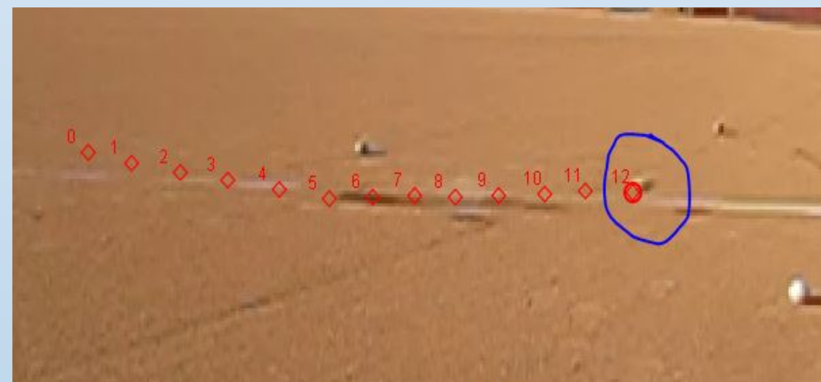
Figure 4: Tracker location of the ball (red marks) over a sequence of video frames, overlaid on the last frame. The ball is highlighted with the blue circle. In each measurement, at least five frames were used both before and after the impact with the ground.
