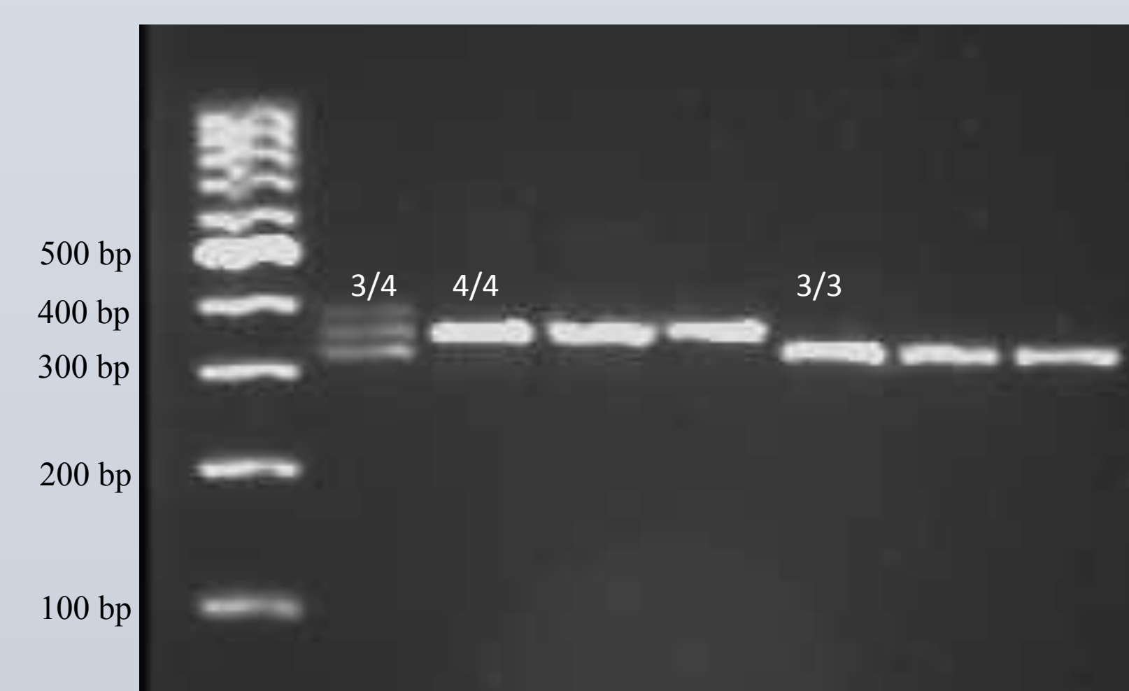
Figure 2. Gel showing a 3/4 VNTR genotype with three bands between 300 and 400 bp, a 3/3 VNTR genotype band at 324 bp, and a 4/4 VNTR genotype band at 354 bp
