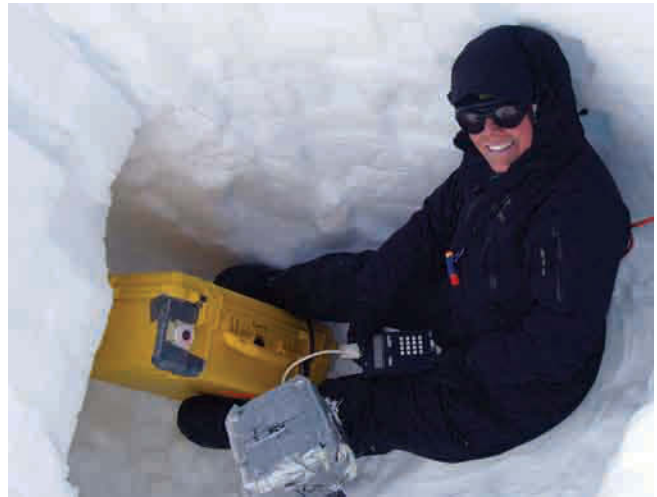
Lora Koenig '99 uses a radiometer to measure microwave emission of the snowpack. The measurements are used to validate space-borne satellite measurements of ice sheets.
