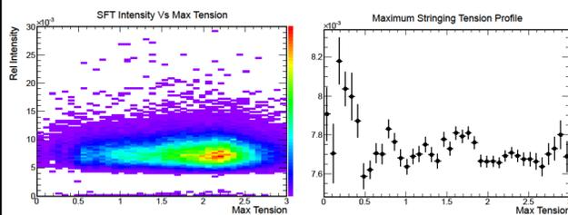
Figure 3. Two dimensional histogram and profile of ratio of transmitted light and maximum stringing tension are shown. The profile shows the mean of each x (x=bin size) Newton bin with error bars indicating a 1 sigma deviation from the mean.
