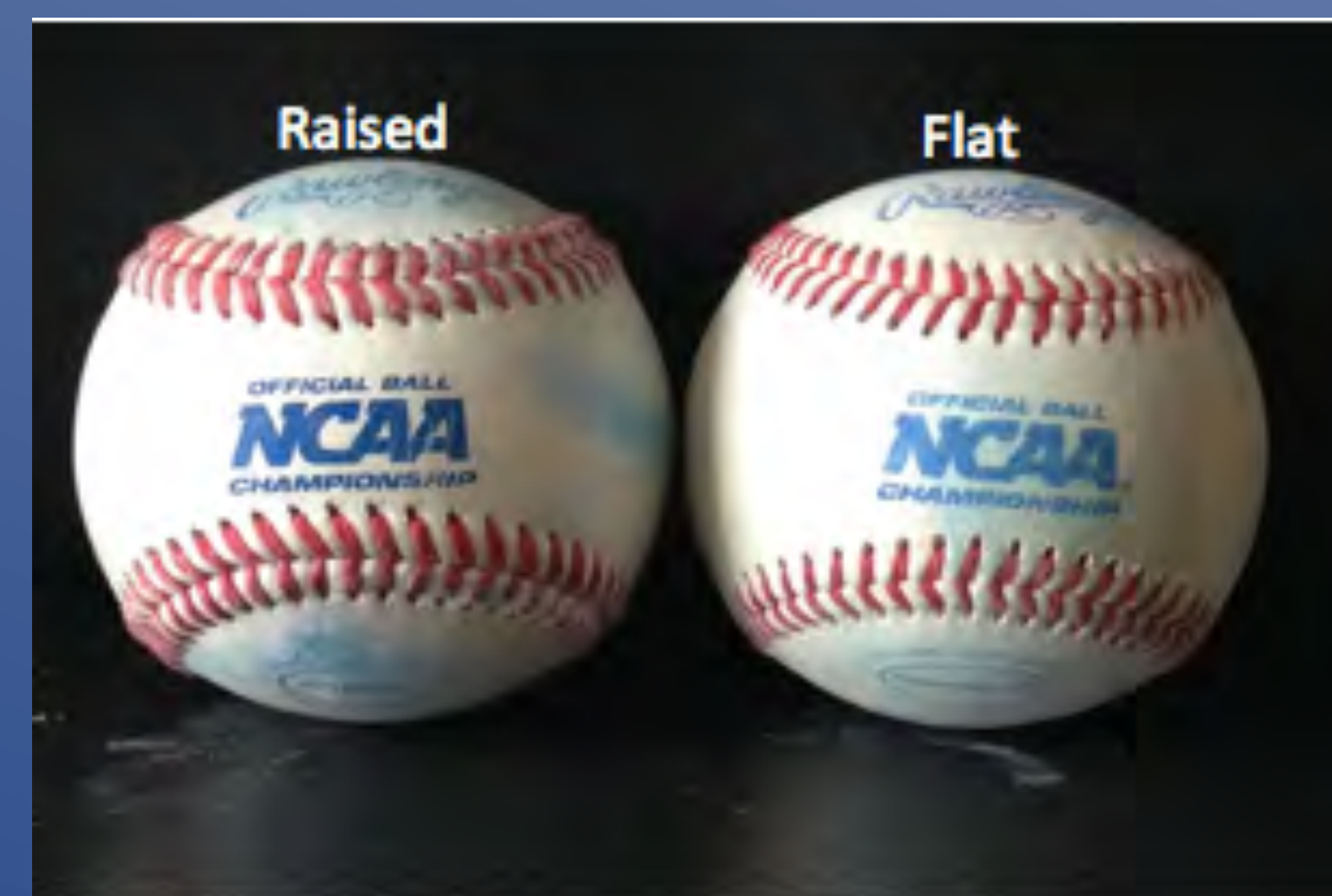
Figure 3.3: Side-by-side comparison of the raised and flat-seam baseballs with seam heights of .048 and .031 inches respectively. Studies done by WSU and Rawlings concluded that flat-seam balls travel greater distances, but there has yet to be a study of their affect on curveballs.
