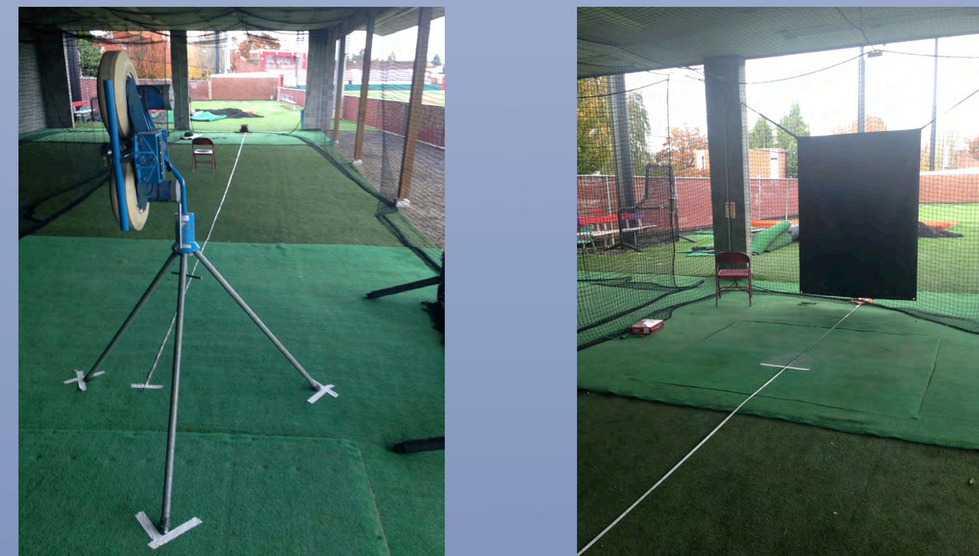
Figure 3.1: JUGS Curveball Pitching Machine. The top wheel spins faster than the bottom wheel, according to recommended settings in the pitching machine manual, which results in realistic curveballs of any desired velocity [2]
