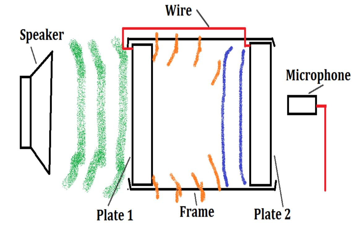
A microphone was used to collect sound waves which passed through the plates in order to determine the effectiveness of the sound damping. The plates were wired so as to separately test the piezoelectric effect (sound absorption) and the converse effect (production of the new wave), and isolate these from other effects which may have contributed to noise reduction. Sound frequencies from 100 to 2000 Hz were tested.
