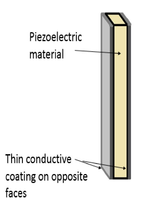
In this system, some sound is expected to make it past the first plate. The energy absorbed by this plate is sent as an electric signal to the second plate. The second plate uses this to output a new sound wave in order to cause destructive interference between the plates.
