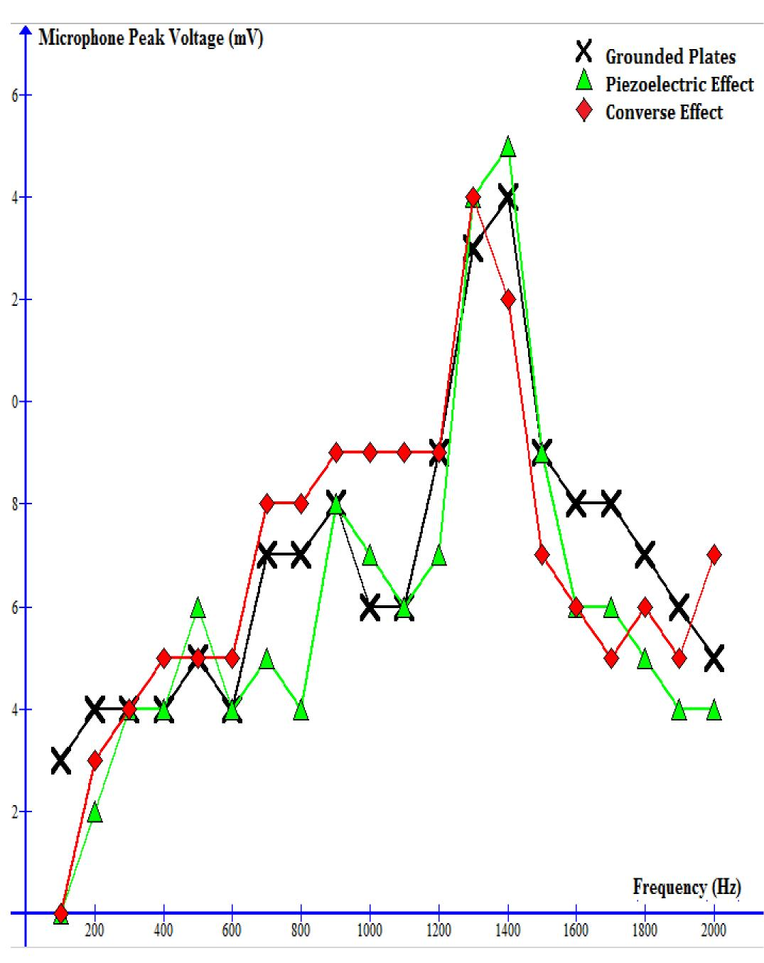
The signal received by the microphone while testing the piezoelectric effect was generally smaller than when the plates were grounded, as expected.
