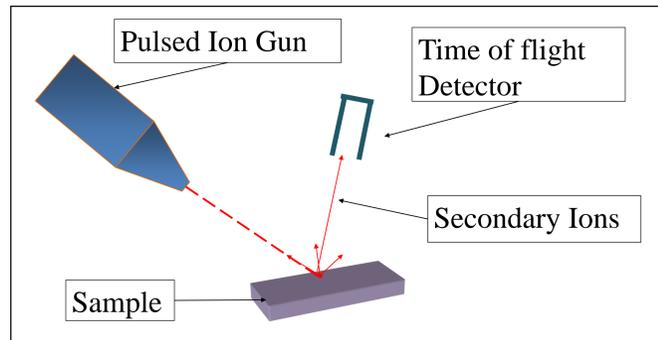
Figure 3 Schematic of a typical TOF-SIMS system..
