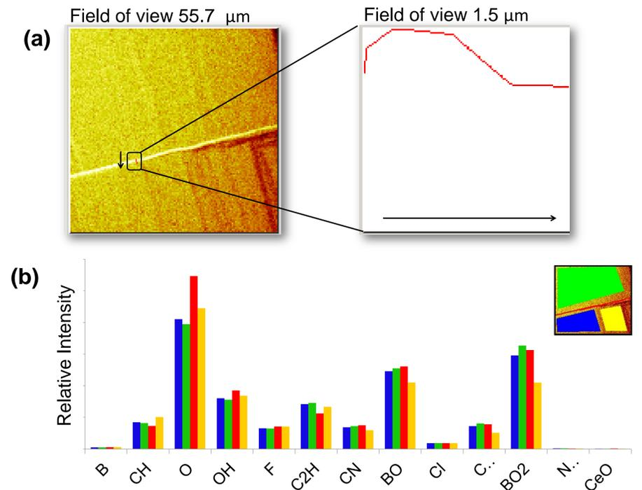
Figure 6: (a) Map of the TOF-SIMS signal strength for O<sub>2</sub>. (b) Signal strength for each prominent peak in the spectrum, for distinct regions of the image. The regions and color scheme are indicated in the inset. These data are normalized by the total ion signal in that region. This helps distinguish true differences in composition from effects that increase overall ion yield (such as topographic features).
