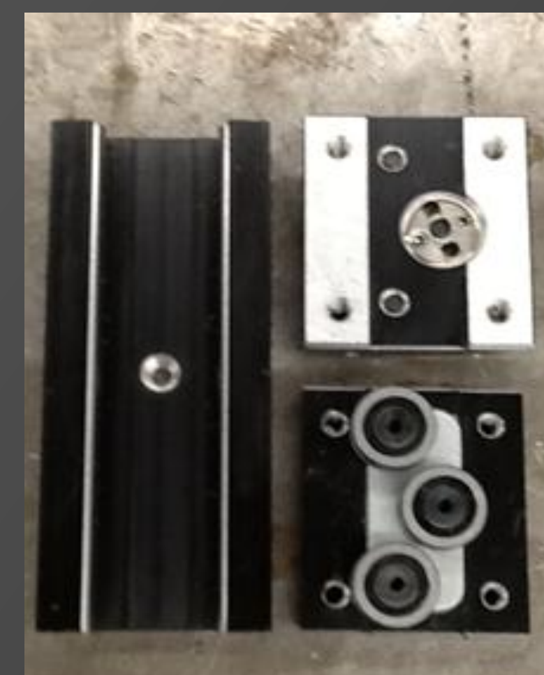
The linear track and block used to guide the directions of motion
