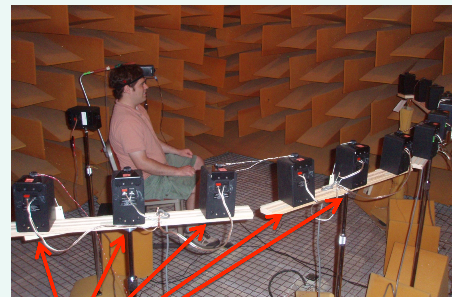
Figure 3. Listener seated in the anechoic room with 90° array of real speakers in front two meters away.
