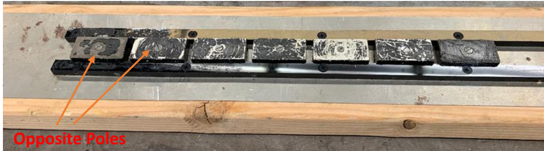
Figure 5: Seven permanent magnets on the stator with alternating poles.
