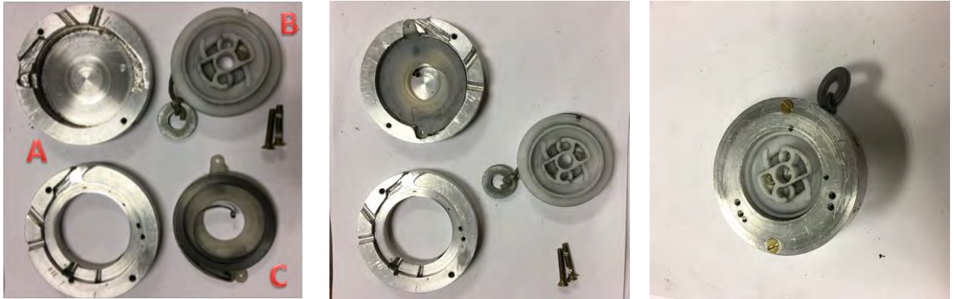
Figure 2.1 Mechanical assembly of string pulley system. (a) Individual components: A. housing unit, B. rotor, C. spring. (b) Spring put into the housing unit. (c) Pulley string components put together
