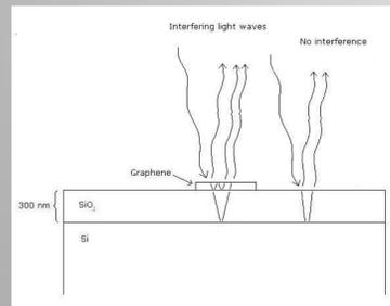
Fig 2: Diagram comparing light shone on graphene and light shone directly on the surface of  $\text{SiO}_2$ . The interference caused by graphene creates a slight contrast between the graphene sample and the bare substrate.
