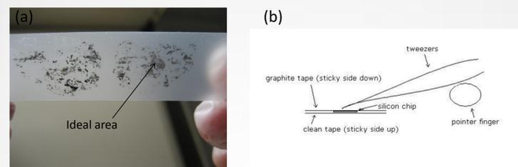
Fig 4: (a) A piece of tape with thin milky-gray graphite deposits, ideal for creating graphene. (b) A schematic for how to transfer graphite and graphene from tape to the silicon chip. The back end of the tweezers is used to lightly rub the tape against the chip.
