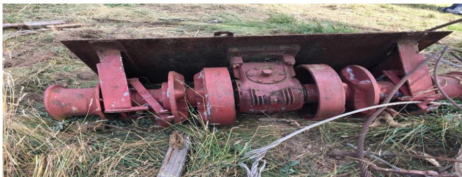
The rusty hydraulic capstan as it sat in the City of Glen Cove department of public works yard in early October 2017. Photo by Vinny Martinez Jr.
