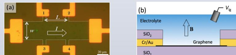
**Figure 1.** a) Hall bar geometry showing direction of current. White lines highlight geometry of graphene. Measurements of V<sub>xx</sub> are measured from terminals 1 and 2; V<sub>H</sub> from terminals 1 and 3. b) Schematic of cross section of device. A tungsten probe provides gate voltage
