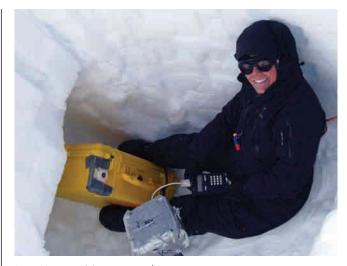
Lora Koenig '99 uses a radiometer to measure microwave emission of the snowpack. The measurements are used to validate space-borne satellite measurements of ice sheets.
