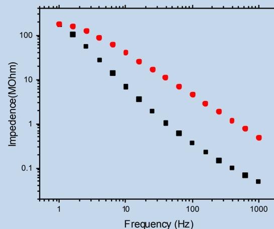
Figure 5. Model of our system on a graphene device. Imaginary impedance is modeled as a capacitor (red) and real impedance is modeled as a resistor (black).
