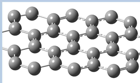
Figure 1. Atomic structure of graphene
