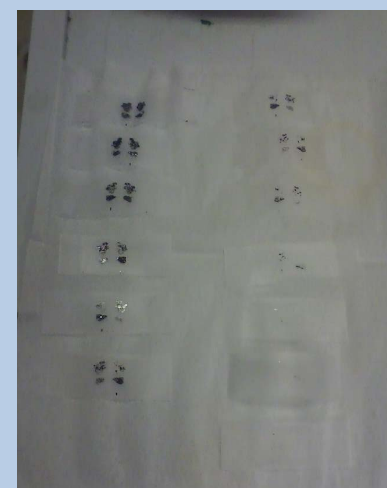
Figure 6. Graphene and graphite on tape during mechanical exfoliation.
