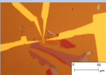
Figure 11. Final device, after lift off.
