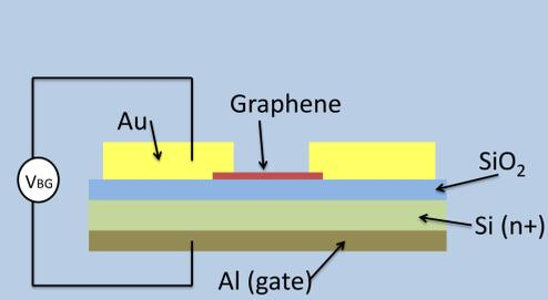
Figure 2. Schematic – Device side view
