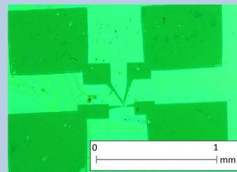
Figure 10. Gold is thermally evaporated.
