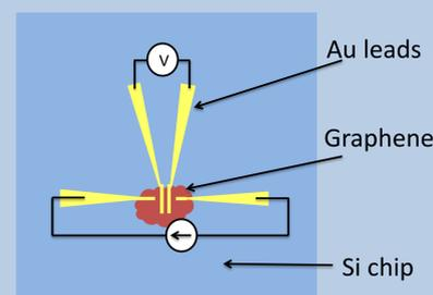
Figure 3. Schematic – top view (graphene leads)
