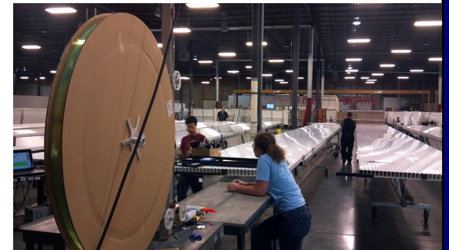
Figure 5. A photograph of fiber stringing at the NOvA module factory, located in Minneapolis, MN. A pulley is used to pull loops of fiber down individual cells. Fibers are shipped to Minnesota on spools (left).
