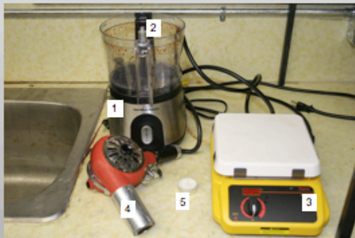
Fig. 1: Photograph of a modified food processor (1) with platform (2), hot plate (3), hot air gun (4) and candle wax (5).
